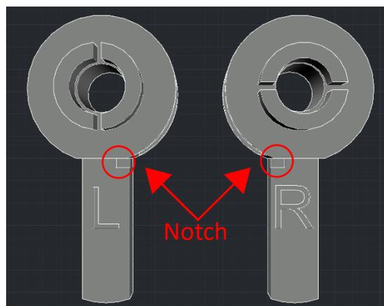
1. The DRL has two tabs on its base, one large and one small. Align the bulbs such that the large tab is on the same side as the notch on the key.
